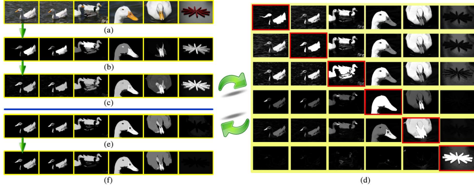
Fig. 1. The framework of our co-saliency model. The red box in (d) represents the query image and each row presents corresponding ranking results. (a) Input image set (b) Single image saliency map (c) First stage guided detection results (d) Second stage guided detection results (red: query) (e) Fusion results (f) Final co-saliency maps.
