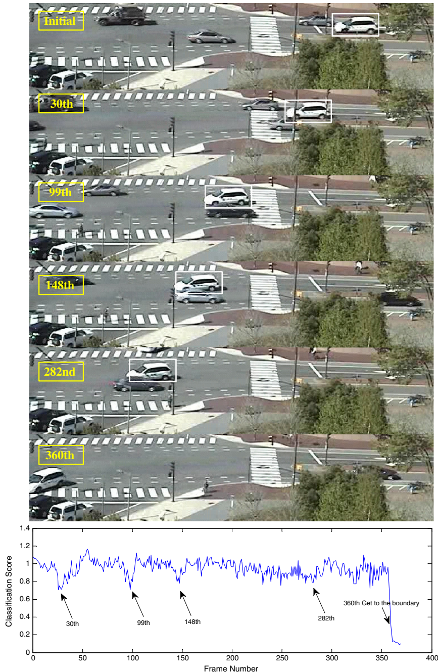
Fig. 9 Tracking score of the whole tracking process. In this sequence, a white car is tracked by our one-class SVM tracker (OCST) method. When the target is partially occluded by other objects, the curve drops down to some level, but comes back in a short time. When part of the target disappears near the boundary of the scenario, the score curve drops enormously and never comes back.
